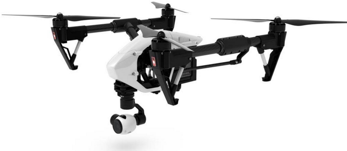
FIGURE 2: VENTUS’S INSPIRE 1 WITH BUILT IN VIDEO/CAMERA SYSTEM
