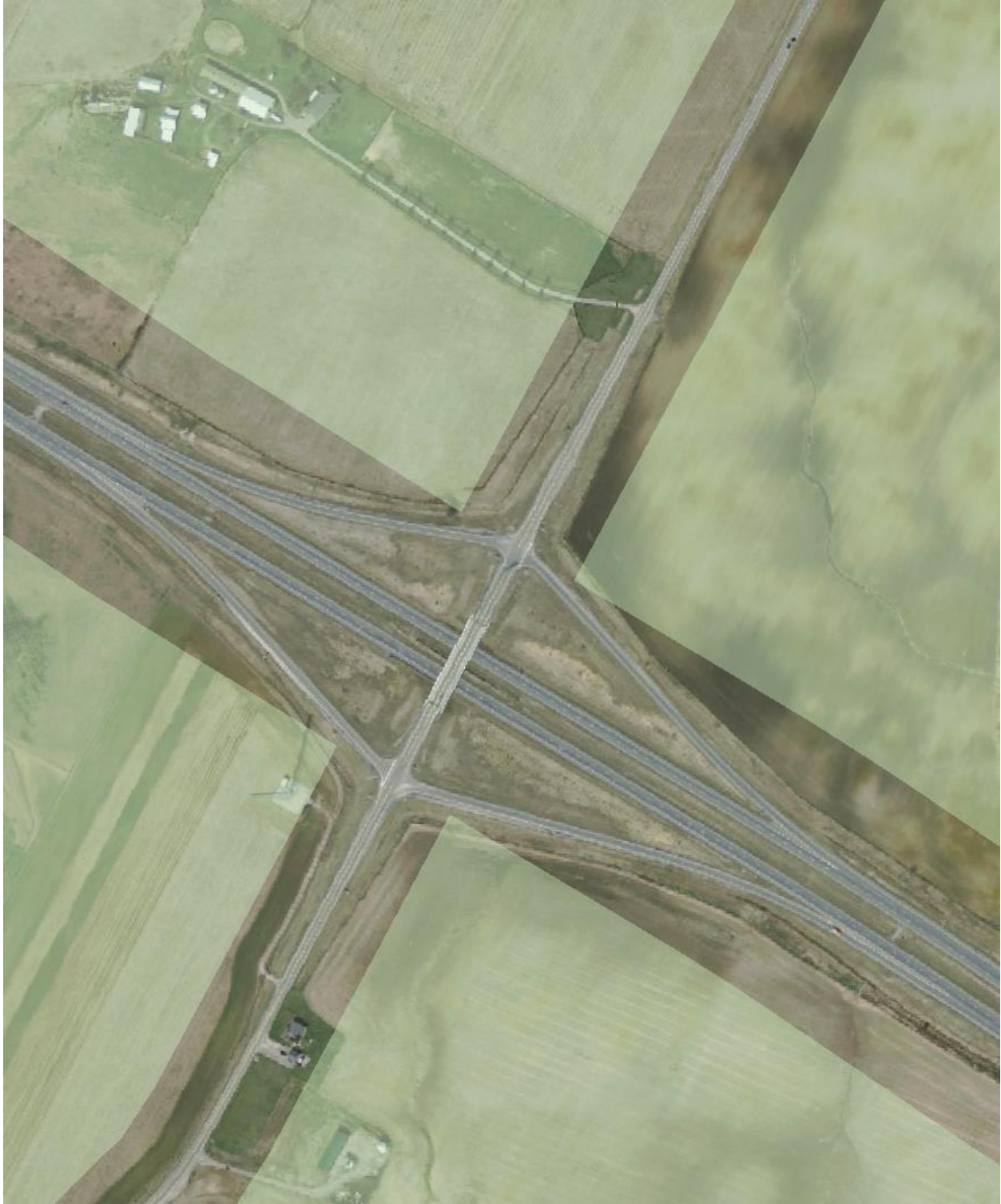
Figure 4: Example of a flight exclusion zone of 100 meters around a state road with more than two lanes, and a 50 meter flight exclusion zone around a state road with two lanes or less.
